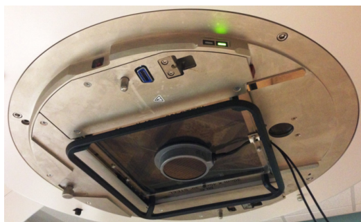
Fig. 1. The Stealth Detector (IBA Dosimetry) is attached to an interface plate which is securely slid into the interface mount of the Varian TrueBeam (Version 1.6).
